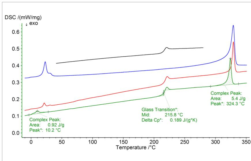
**3a** Comparison of the DSC curve of an unknown polymer (green) with the most similar database curve (red, measurement of "PEI-PTFE Luvocom 11067223", see figure 3b), and with typical database curves for PTFE (blue) and PEI (black). The curves were staggered in the y-direction for better illustration.
