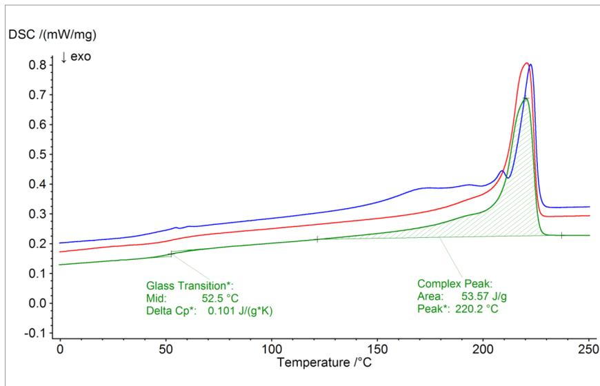
**2a** Comparison of the DSC curve of an unknown polymer (green) with the most similar database curve (red; measurement of "PA6 Altech PA6 A 2030-109 GF30") and the database curve of "PA610 Terez PA610 GF30 H ECO" (blue), see figure 2b.
