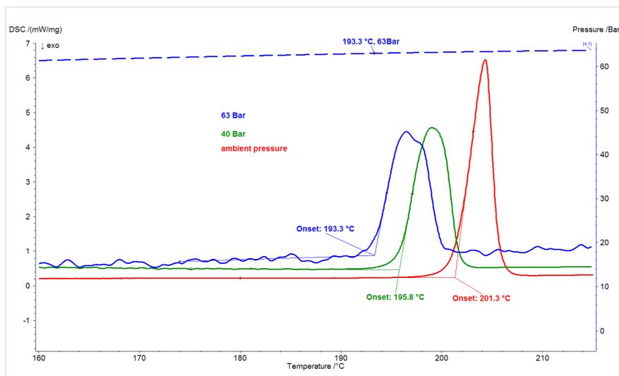
1 DSC thermogram of piroxicam form I (10 K/min) under CO<sub>2</sub>
