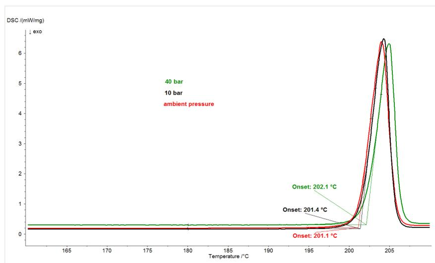
2 DSC thermogram of piroxicam form I (10 K/min) under N<sub>2</sub>
