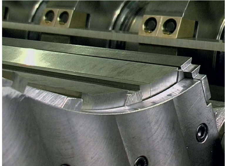
Stator knife assembly in housing side part
