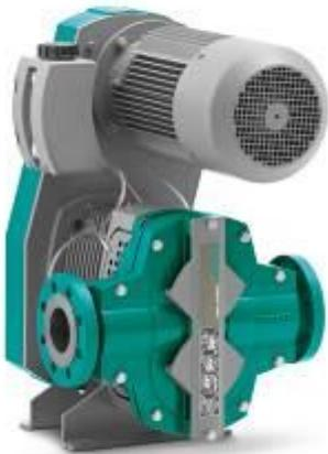
The positive displacement pump is suitable for sticky and dry substances, thixotropic, dilatant, shear-sensitive and abrasive media with viscosities of 1 to 1,000,000 mPas. Depending on the size of the system, up to 1,000 m<sup>3</sup> can be pumped an hour.
